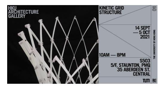
Advances in architectural geometry and mechanical simulation have revealed a new kind of spatial mechanism that can be constructed from straight elastic lamellas connected through scissor joints. These lamella grids can be easily manufactured and offer a controlled movement from a flat shape into a doubly curved shape, with the potential to inform the design of transformable structures at all scales, ranging from foldable roofs and adaptive building facades to medical stents for heart surgery.
